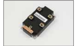
Insulated Gate Bipolar Transistor (IGBT). Rated 4,500 Volts, 900 Amps.
